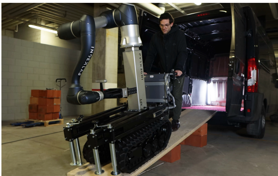
Figure 12. Unloading the Bric-a-Brick is a simple and straightforward process involving just one person. Using a normal construction site three-layer laminated spruce panel for formwork reinforcement, an operator creates a slope to unload it from the van and manually guides it to the location on site.
