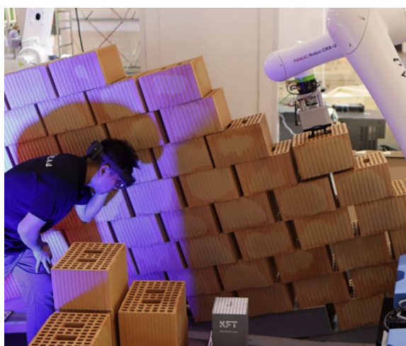
Figure 6. The BRIX prototype in action at 2023 SAIE Construction Fair in Bari, Italy. This manufacturing system designed for on-site construction uses a rover and a robotic arm that work collaboratively with construction workers, who use augmented reality Microsoft HoloLens2 for improved supervision and safety management. This integration highlights the effective combination of human skills and robotic efficiency in construction.
