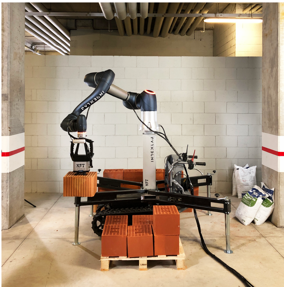
Figure 16. The first tests of pick-n-place of Bric-a-Brick performed at INDEXLAB, Lecco.
