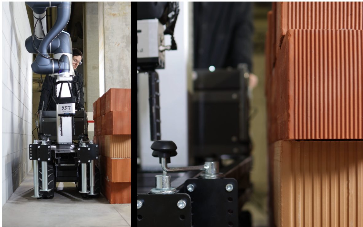
Figure 10. Photo of Bric-a-Brick passing through a 800 mm passage. The wheelbarrow and the retracted stabilizing system account for around 600 mm of the total width, while the robot in pack position adds another 100 mm.
