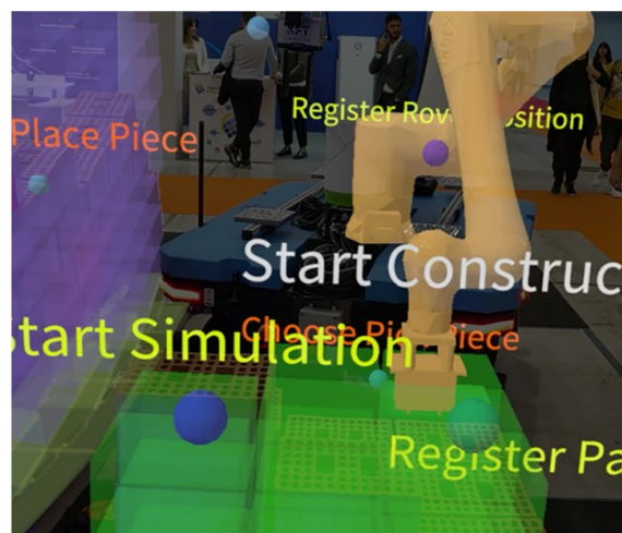
Figure 6. The BRIX prototype in action at 2023 SAIE Construction Fair in Bari, Italy. This manufacturing system designed for on-site construction uses a rover and a robotic arm that work collaboratively with construction workers, who use augmented reality Microsoft HoloLens2 for improved supervision and safety management. This integration highlights the effective combination of human skills and robotic efficiency in construction.
