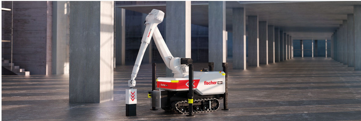
Figure 2. Fischer's Baubot is an automatic fastening robot which is used in combination with a digital BIM construction plan. It is an industrial robot on a vehicle with tracks that is meant to automate large construction site processes involving drilling and fastening, but since it is very heavy for small-scale construction, it needs specific use-cases to be successfully employed.
