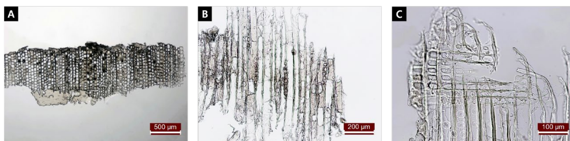
Figure 3. Micrographs of Hard Pine (A) Cross section( \times 40 ), (B) Tangential section( \times 100 ), (C) Radial section( \times 200 ).
