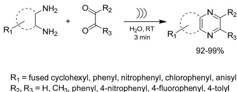
**Figure 3.** General Synthetic Route for the Ultrasound-Assisted Preparation of Benzopyrazine Derivatives.
