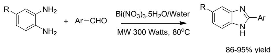
**Figure 2.** General scheme for the synthesis of benzimidazoles using microwave irradiation and bismuth nitrate pentahydrate-catalyzed reaction [22].
