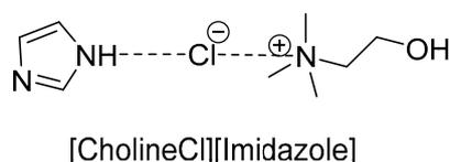
**Figure 6.** Proposed formation of a deep eutectic solvent (DES) between CholineCl and IM via hydrogen-bond interactions [75].
