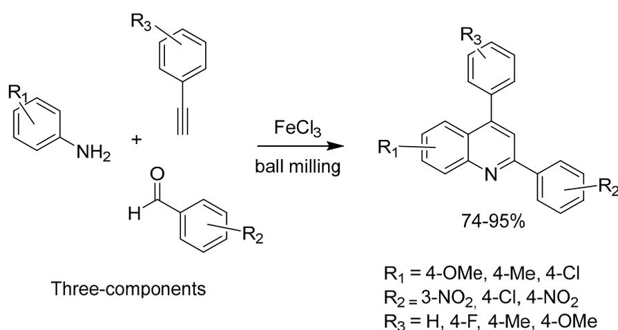
**Figure 4.** General scheme for the synthesis of 2,4-diphenylquinolines via a three-component reaction under ball-milling conditions [68].
