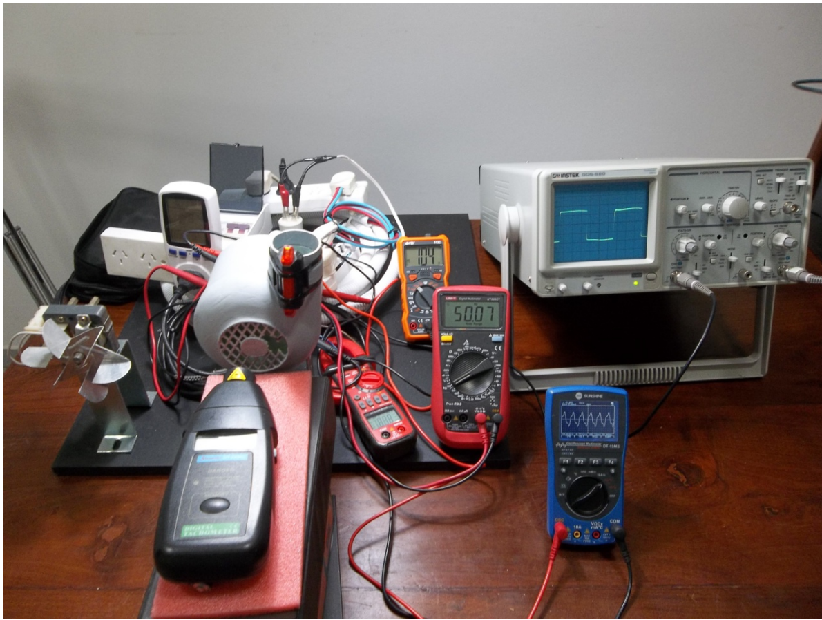
Figure 34. Test bench connected to the SARS-CoV-2 or Covid-19 (Coronavirus) centrifugal extractor/blower motor for stale air: Turbo. With digital multimeter (AC volt meter), clamp meter (AC current meter), frequency meter (Hertz meter), laser photometer (RPM speed meter), digital oscilloscope waveform meter alternating current in voltage ( V_{peak} , V_{avg} , V_{rms} ), for calculating the harmonic distortion crest factor, analog oscilloscope for qualitative observation of the THD (alternating current harmonic distortion), wattmeter (active power meter in watts or watts), power factor (cosine of \phi ), power-meter (active energy consumption meter in kilowatt-hours: kWh). Source: self made.
