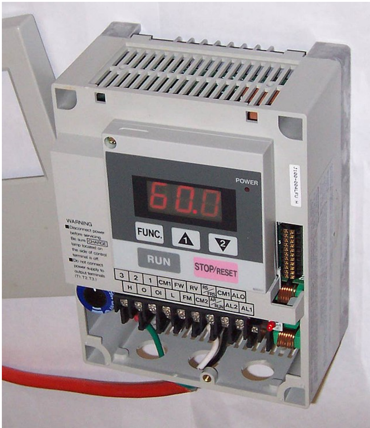
Figure 22. A variable frequency drive (VFD acronym: Variable Frequency Drive or AFD Adjustable Frequency Drive) is a system for controlling the rotational speed of an alternating current (AC) motor by means of frequency control power supplied to the motor. A variable frequency drive is a special case of a variable speed drive. Variable frequency drives are also known as adjustable frequency drives (AFDs), AC drives, or microdrives. Since the voltage (or voltage) is made to vary at the same time as the frequency, they are sometimes called VVVF (Variable Frequency Variable Voltage) drivers. Fountain: https://commons.wikimedia.org/wiki/File:Small_variable-frequency_drive.jpg
