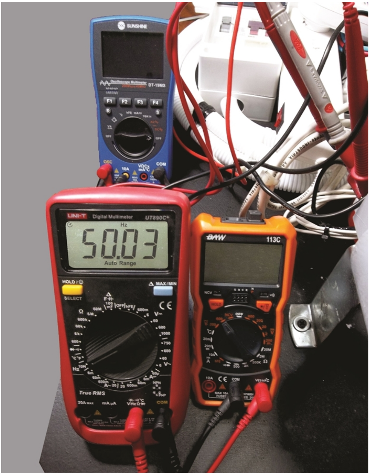
Figure 35. View of the frequency meter turned on indicating 50 (Hertz) of alternating current (AC), together with the digital multimeter (voltmeter) turned off. Source: self made.
