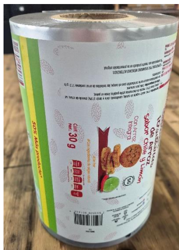
Figure 1. A laminated coil is used to form flexible packaging with different plastic films.
