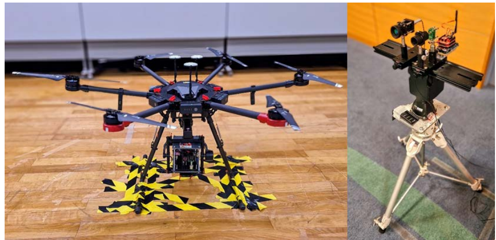
Figure 2. Drone with mounted Lasercom Module and an ad-hoc optical receiving system.
