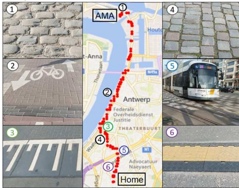
Figure 8. Journey of ca. 5.5 km from AMA to home by bike at an average speed of 11 km/h together with the position of the events caused by irregularities in the road. The red dots stand for cyclist's position according to the GPS sensor GY-GPSV3-NEO-M8N.
