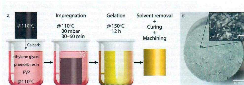
**Figure 15.** a) Processing steps for near net-shape samples of HARLEM. b) Frontal view of a HARLEM sample with density of 0.27 g/cc. Optical microscopy image featuring the resin-containing phase within the carbon fibers (inset) (Reprinted from [28]. Copyright by the authors).
