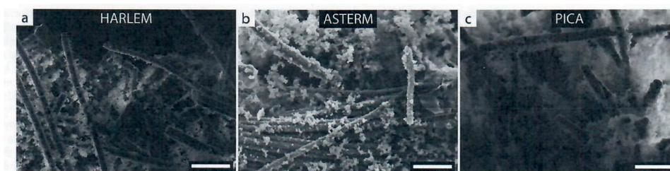
**Figure 16.** Electron Microscopy images of the carbon-phenolic ablators (a) HARLEM, (b) ASTERM, and (c) PICA. Scale bars: 50 µm (Reprinted from [28]. Copyright by the authors).
