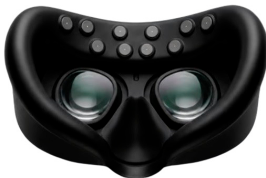
Figure 2. Electrode location on the mask: 8 electrodes are channels and 2 electrodes are reference and bias.
