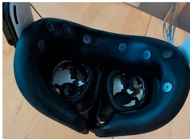
Figure 3. General view of the first Mask prototype with integrated silver/silver chloride electrodes.
