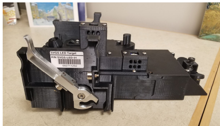
Figure 1. Integration of the SVGS beacon with NASA's Astrobee free-flying robot using the M561 payload interface. The SVGS beacons can be mounted either on the robot payload bay or on ISS structural elements, enabling multiple experimental configurations.
