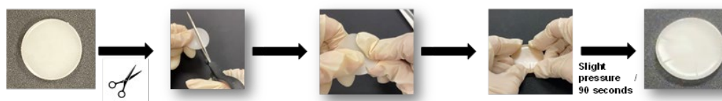
Figure 6. Scheme of the intrinsic self-healing test performed in PU discs. The process involves (from left to right): initial specimen; partial cut of the disc; re-joining of the cut pieces; manual pressing for 90 seconds; and final healed PU.
