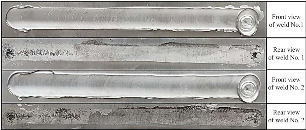
Figure 25. Forming surface of weld under constant pressure control.
