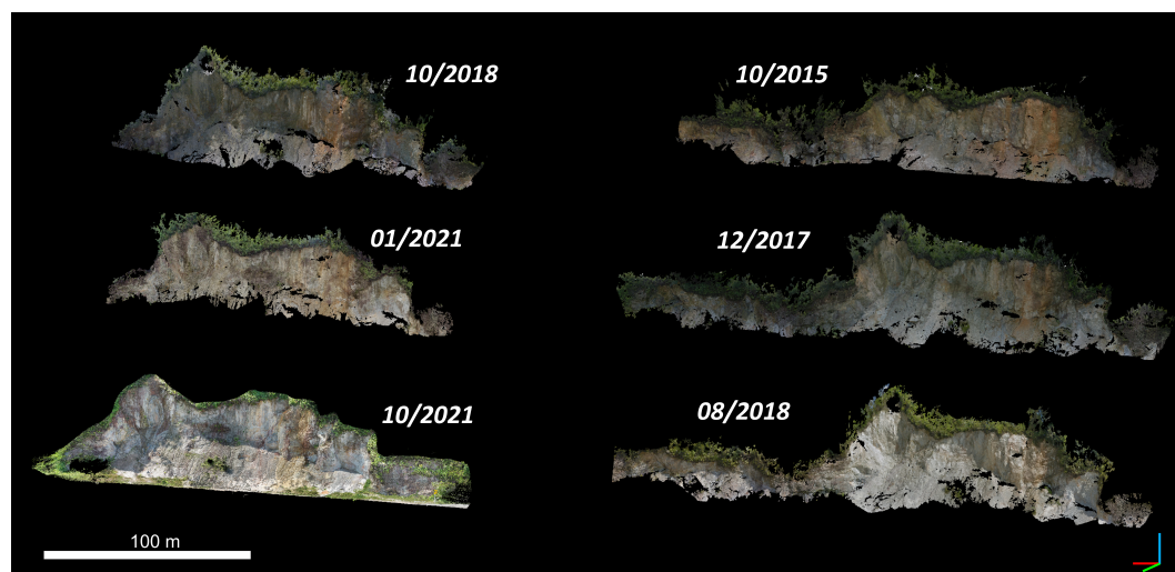
Figure 6. Result of SfM for 7 years of SVI data from 2015 – 2021. The 3D point clouds from 10/2015 to 01/2021 are resulted using images from SVI and 10/2021 are result from UAV acquisitions.
