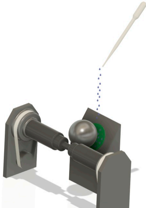
Figure 1. Schematic representation of the operational principle of the ball-cratering wear test.
