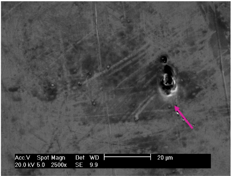
(e) Corrosion pits formed on a non-marked (blank) specimen after cyclic polarisation test.
