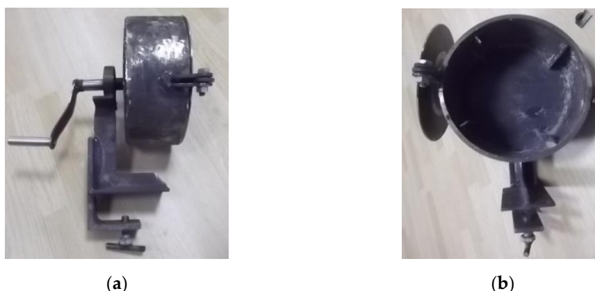
Figure 4. Drum for testing abrasion of briquettes subjected to thermal shock.
