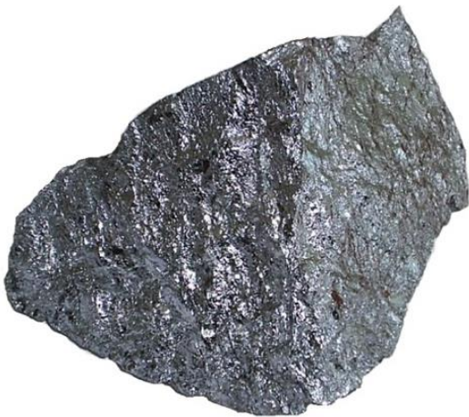
Figure 12. Fracture of a technical silicon ingot.
