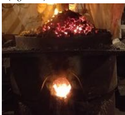
Figure 11. Smelting of metallurgical grade silicon using briquettes.
