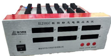
Figure 6. XL2101C static strain gauge.
