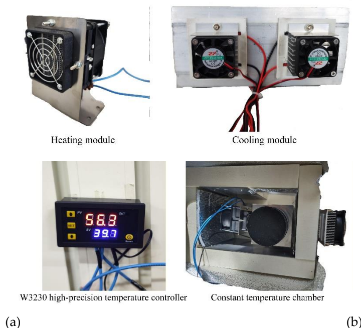
Figure 5. Temperature control system. (a) Heating and Cooling module. (b) Constant temperature chamber.
