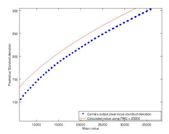
**Figure 3.** Camera output pixel value standard deviation as a function of mean pixel value under constant illumination. The calculated curve indicates that the equivalent full well capacity (FWC) is close to 23000.
