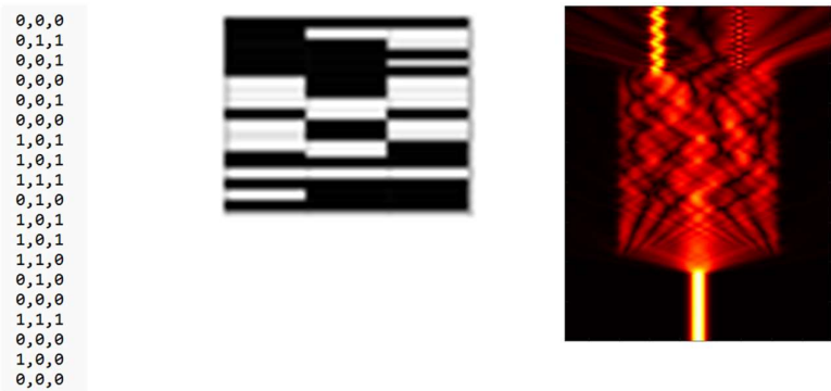
Figure 6. Simulation output in three different formats, straight numerical, B&W graphical representation of the matrix, internally generated EM field.
