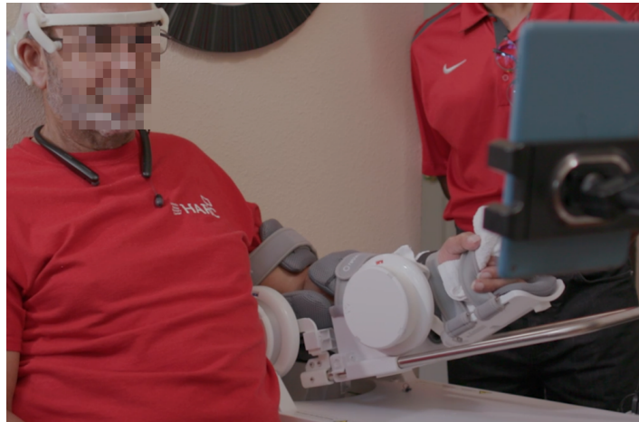
Figure 2: A custom EEG-based BCI headset, with wireless tablet-based graphical user interface (GUI), and an IOT-enabled powered upper-limb exoskeleton robotic device deployed in a neurorehabilitation application.
