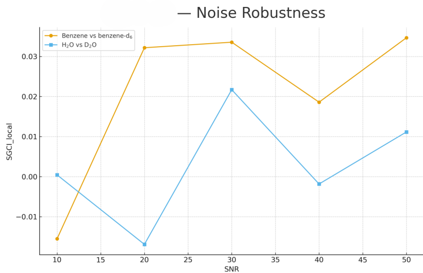
Figure 10. Noise robustness of local SGCI coherence across SNR levels (10–50). Benzene vs. benzene-d 6 maintains stable harmonic coherence, while H 2 O vs. D 2 O shows moderate sensitivity to noise in the high-curvature stretching regions.
