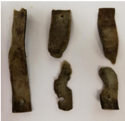
Figure 9. Leather pieces shown in Figure 13B were composted in a 2 L vessel for 44 days.
