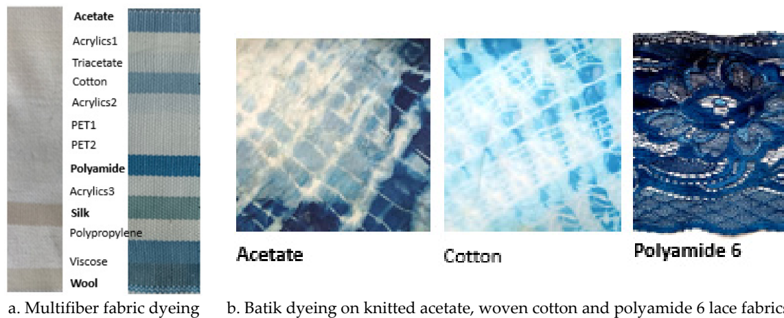
Figure 5. Dyeing of fabrics with blue indigo dyes from Indigofera Persicaria tinctoria , at 50\text{ }^{\circ}\text{C} .
