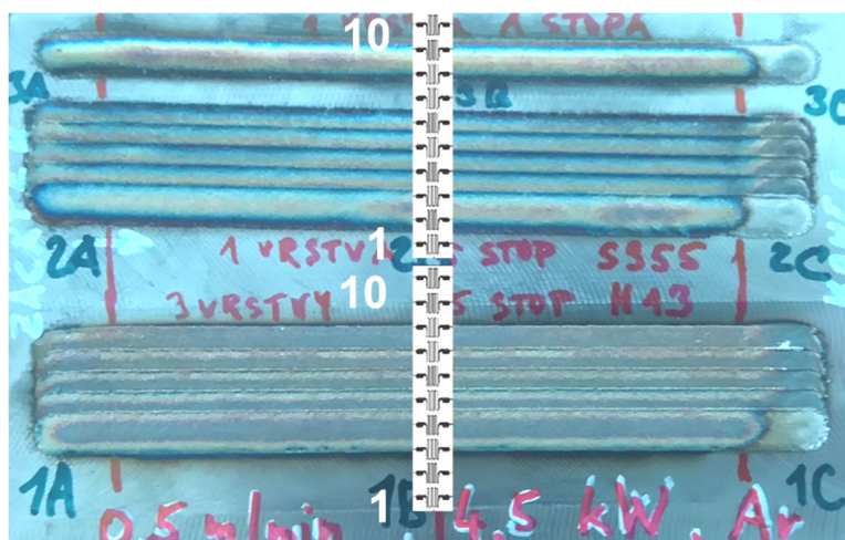
Figure 3. Position of strain gauge chains on the specimen.
