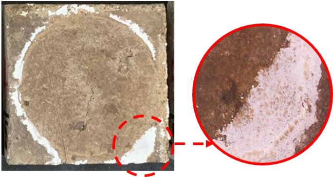
Figure 16. Digital microscopy (Detail chemical attack N.04 – Lactic Acid).
