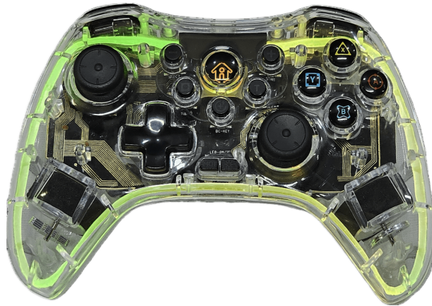
Figure 6. Physical controller used for the teleoperated navigation of the robot.
