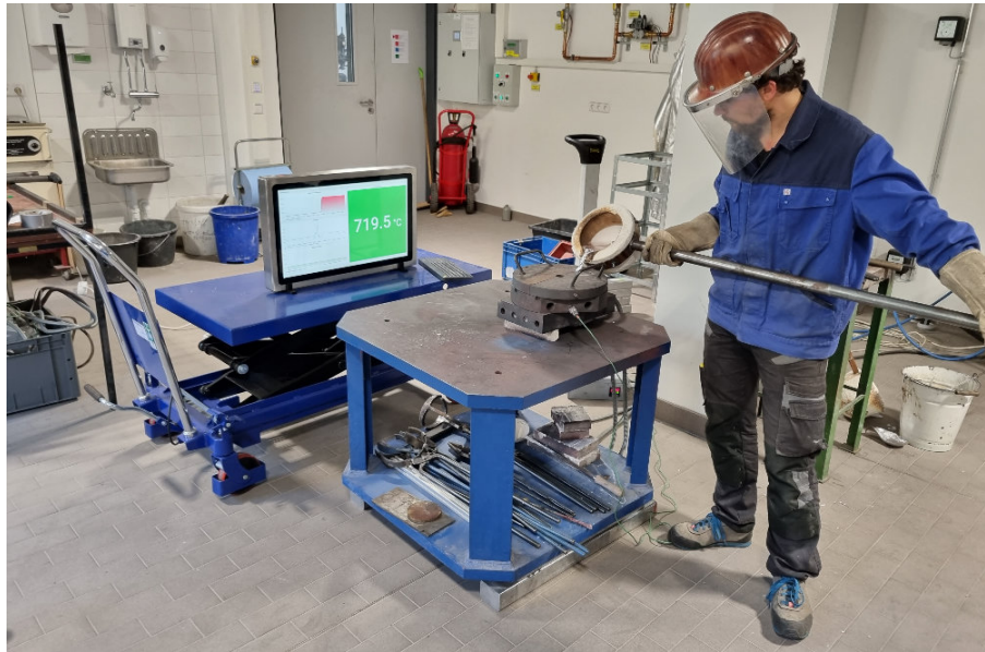
Figure 7. Experimental testing of the sensory infrastructure for recording the relevant process data in manual casting production.
