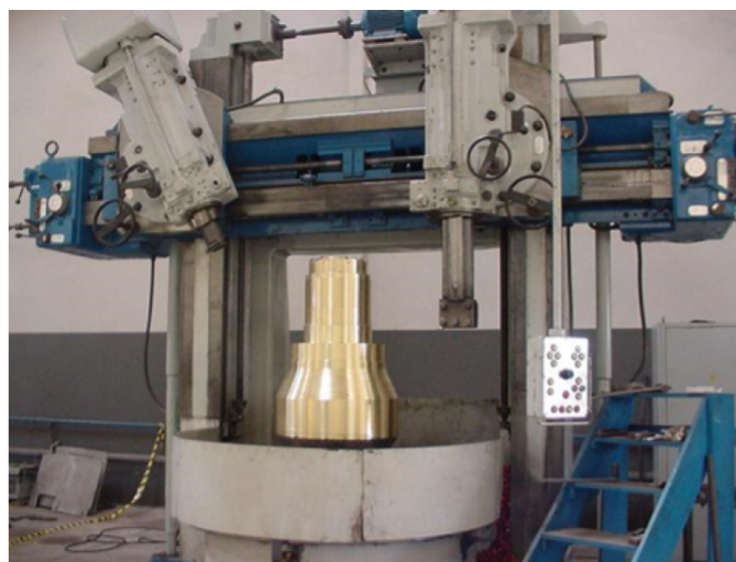
Figure 6. Ingot from which the sphere was machined. Courtesy of Odylio D. Aguiar.
