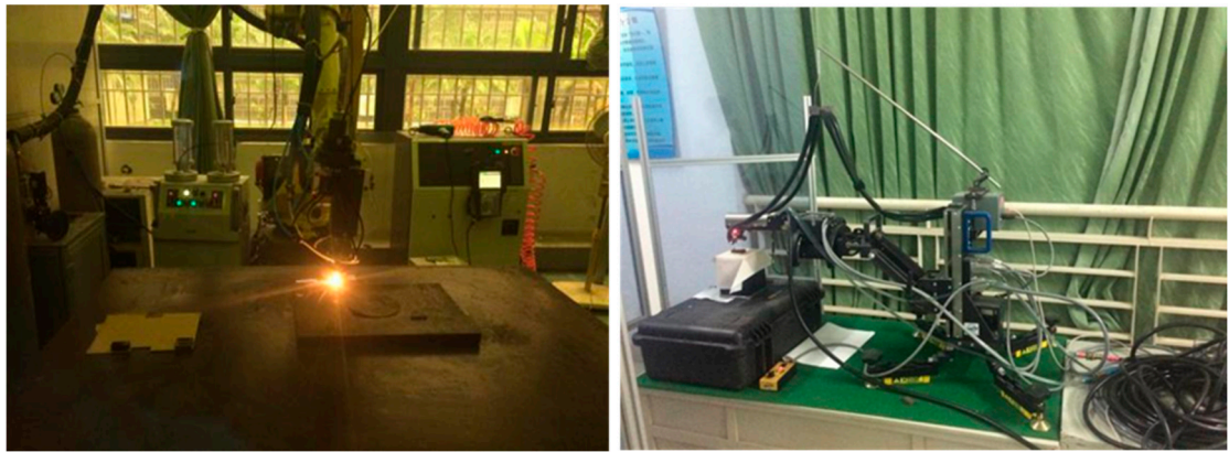
Figure 1. (a) A fiber laser cladding system(b) The tester for residual stresses of Proto i-XRD devices.
