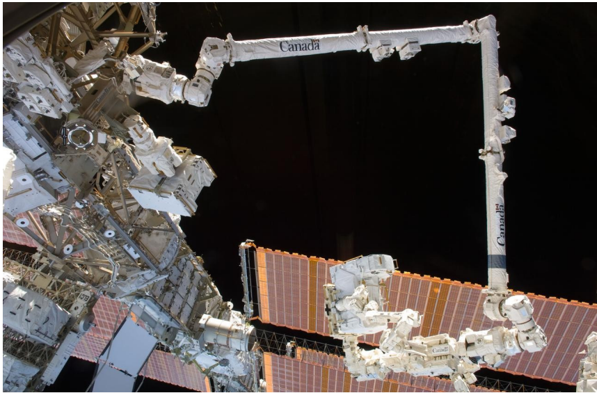
Figure 2. The Canadarm2 (SSRMS) and special-purpose robot Dextre. (Source: https://images.nasa.gov/ ).
