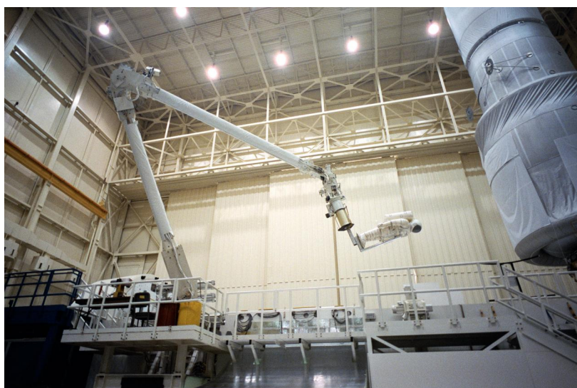
Figure 1. The Shuttle Remote Manipulator System (SRMS). (Source: https://images.nasa.gov/ ).
