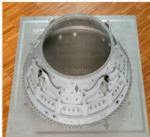
Figure 3. Aerospace component manufactured via metal additive manufacturing using nickel-based alloy Inconel 718 by GE Aerospace, demonstrating lightweight design and consolidated geometry for high-temperature service [37].
