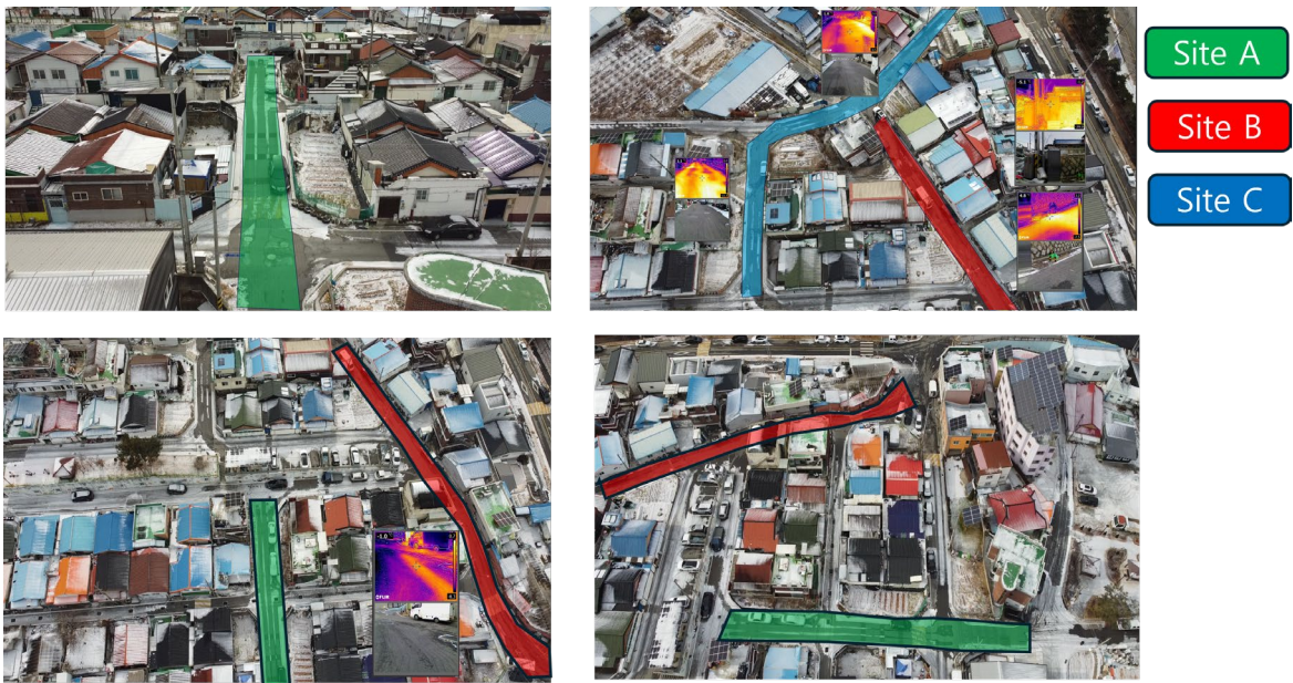
Figure 11. Drone-based monitoring of Sites A–C illustrating differences in de-icing effectiveness.
