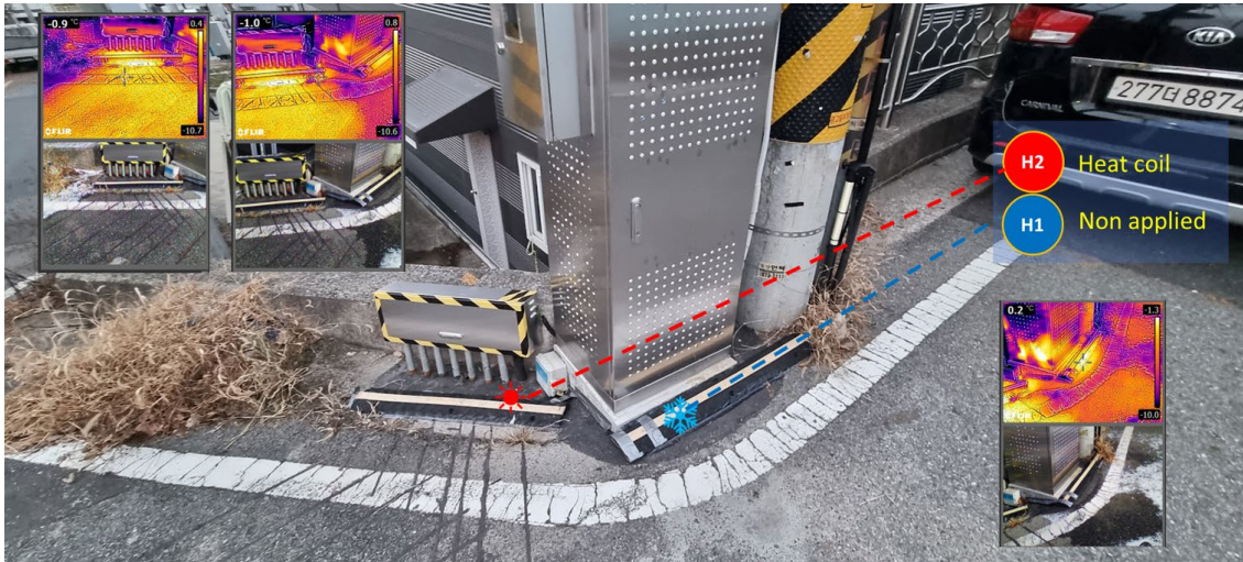
Figure 6. Placement of surface temperature sensors in heated (H2) and reference (H1) sections, with thermal snapshots during RHS operation.
