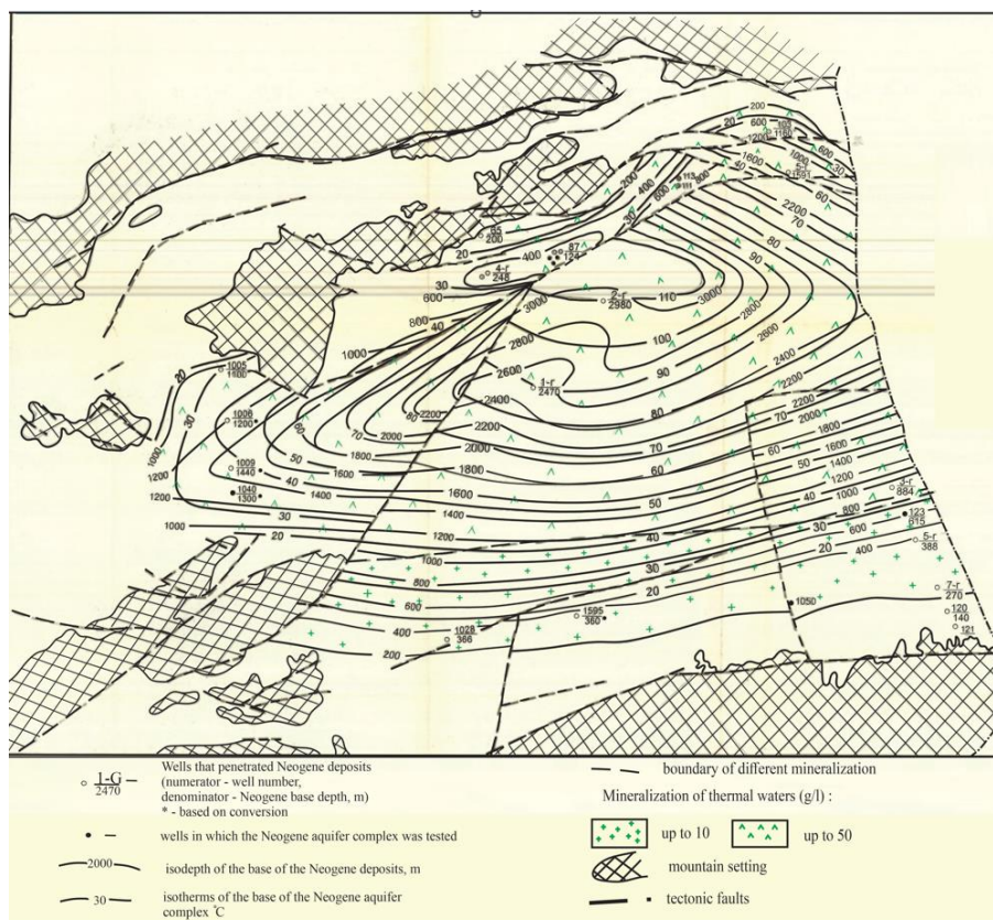
Figure 7. Schematic hydrothermal map of the Neogene aquifer complex in the East Ili trough. [50].
