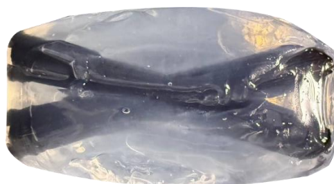
Figure 6. Part based on partially crosslinked sodium alginate with an internal hollow channel after completion of the gelation process.
