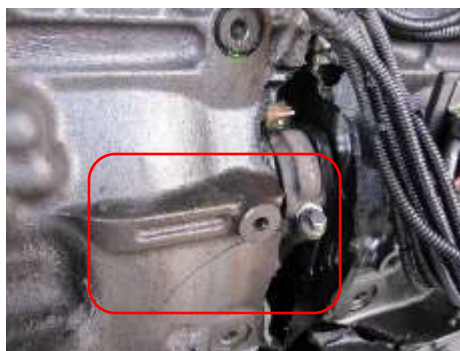
Figure 7. Crack in engine block.
