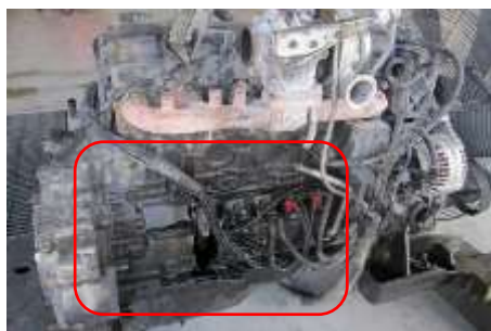
Figure 6. Engine block damage.
