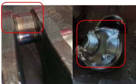
Figure 9. Piston and connecting rod damage.
