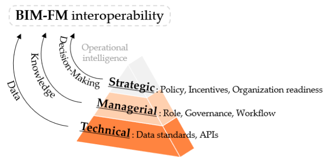
Figure 2 Layered model of BIM–FM interoperability across three dimensions.
