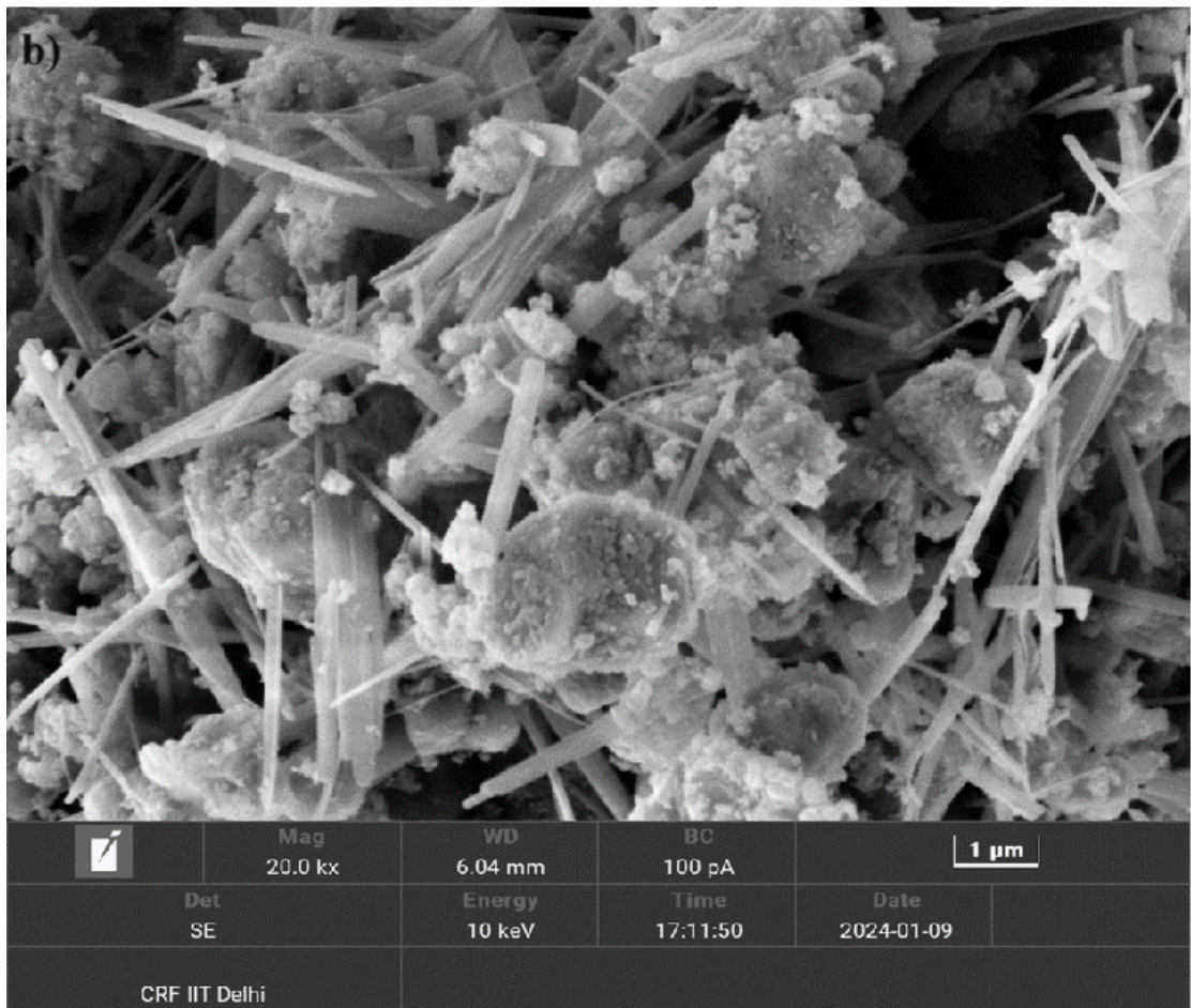
Figure 5. FESEM Sphere like growing alongside nanowires at 1μm resolution.
