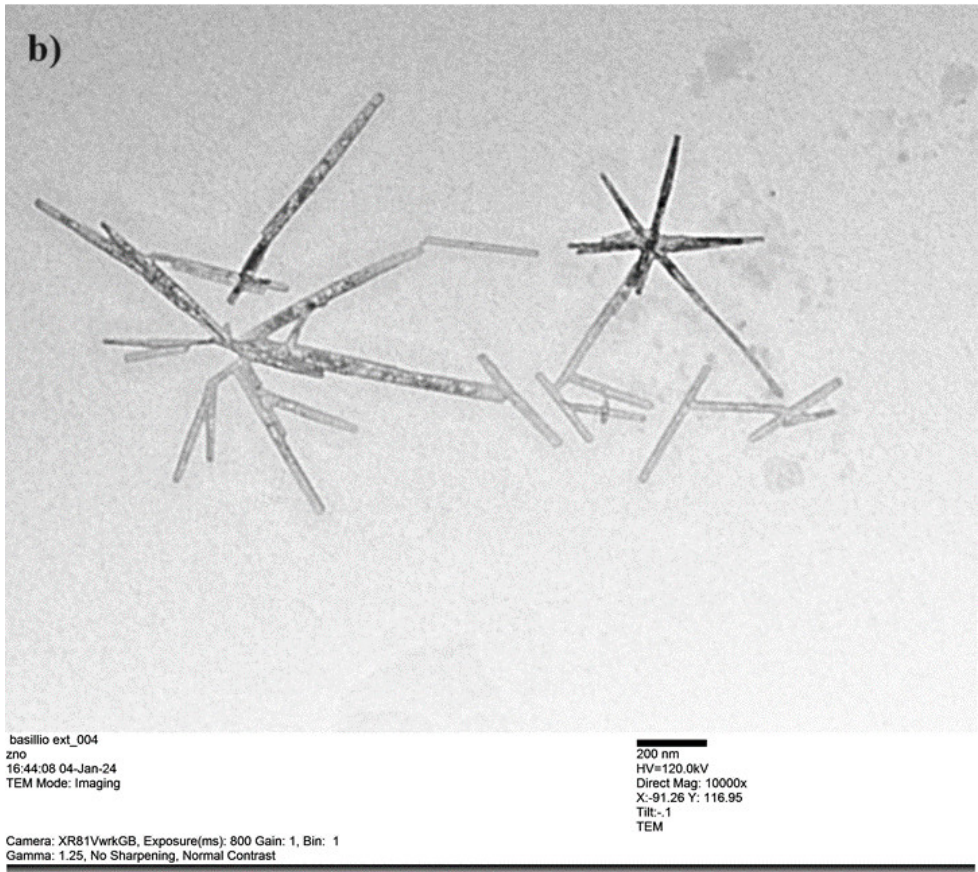
Figure 7. Flower-like Growth Along Wires ZnO Nanoparticles from TEM.
