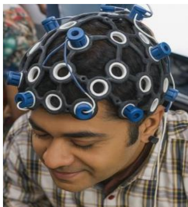
Figure 2. In-House Developed EEG Skull-Cap.
