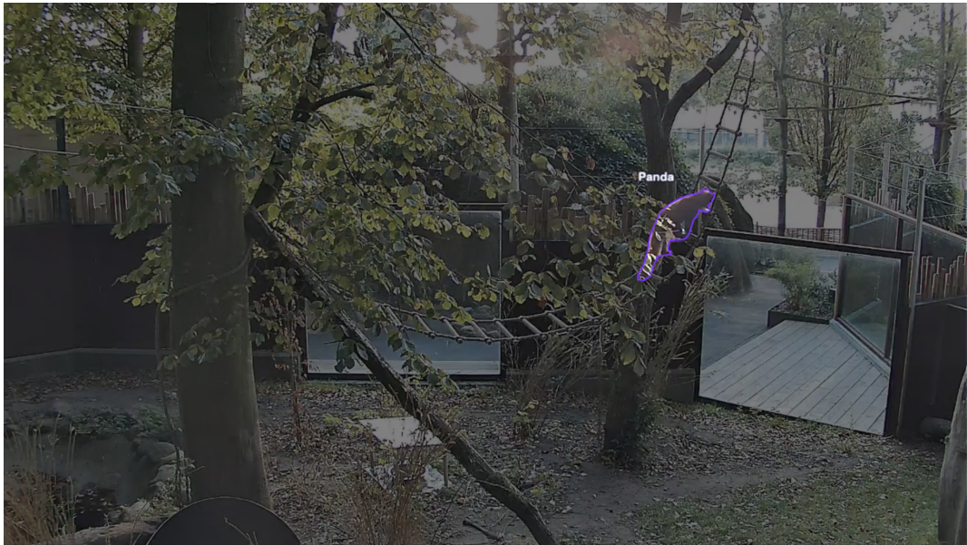
Figure A4. Example of polygon annotation for subject detection. Representative frame from the annotation workflow in Roboflow. The subject is delineated by a manually drawn polygonal mask (purple outline, labelled “Panda”).
