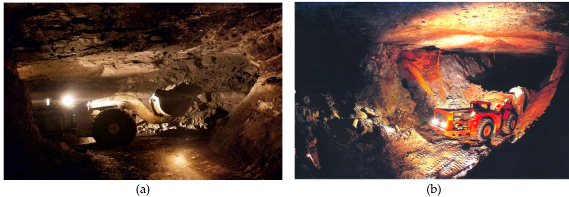
Figure 4. Examples of LHD loader operation in the analysed underground mine: (a) loading and manoeuvring in a low-height drift under constrained visibility conditions; (b) loading of broken ore directly at the production face.
