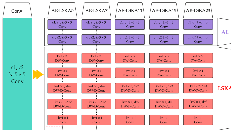
Figure 8. The AE-LSKAs with different dilated kernels and receptive fields.
