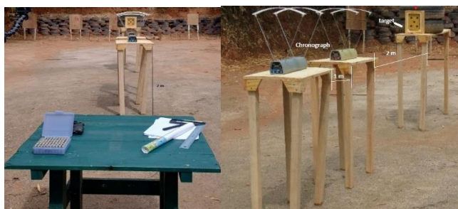
Figure 8. - Ballistic test layout - Arrangement of tables and apparatus.
