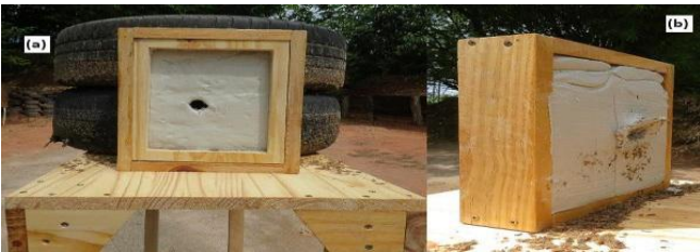
Figure 9. - Ballistic clay after bullet shoot (a) frontal view, (b) posterior view.
