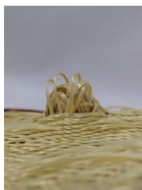
Figure 3. – Simulation of the fabric's deformation in contact with a projectile.
