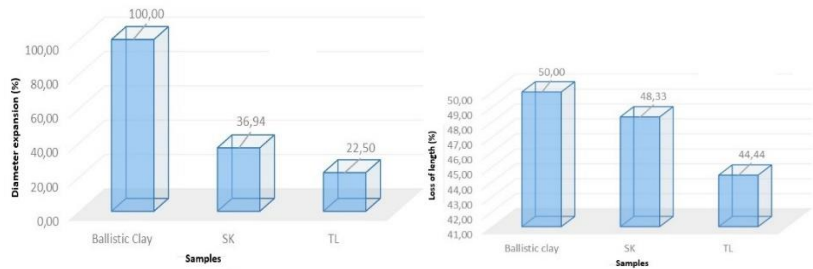
Figure 14. Bullet deformation after impact in relation to the original size (a) and diameter of the projectile (b).
