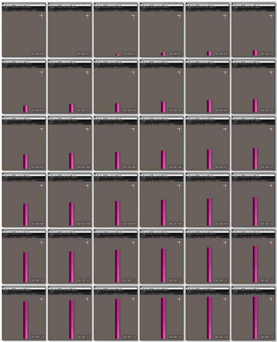
Figure 27. Simulation snapshots of a 100ml volumetric tube filling simulation in Unity.
