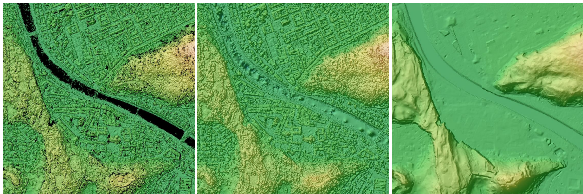
Figure 3. Salzburg, section 1.5 \times 1.5 \text{ km}^2 of the old city-center, left: unfilled DSM derived from the Pléiades triple scene (black=no-data), center: filled DSM, right: reference DTM provided by the state of Salzburg
