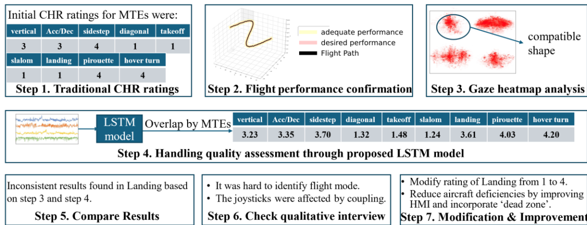
Figure 13. The handling quality assessment process based on the proposed framework.
