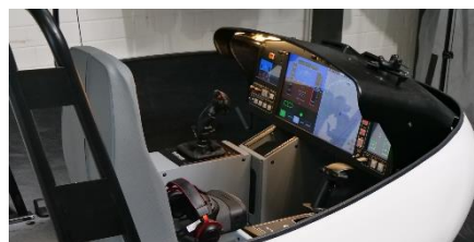
Figure 3. The motion-based mixed reality simulator [32].
