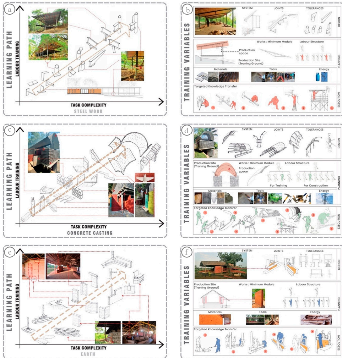
Figure 7. Three examples of on-site capacity-building strategies are illustrated for steelwork (a-b: Ambepussa library), concrete casting (c-d: Kandy sanitary blocks), and earth-based construction (e-f: Farmer field school). The left column of diagrams shows the scaled organisation of building systems by task complexity, creating a skill-building ladder. The right column of images demonstrates how training workshops were organised, showing how systems, joints, and tolerances are 'designed'; production factors are 'planned'; and the steps for execution and training are outlined [23,32].
