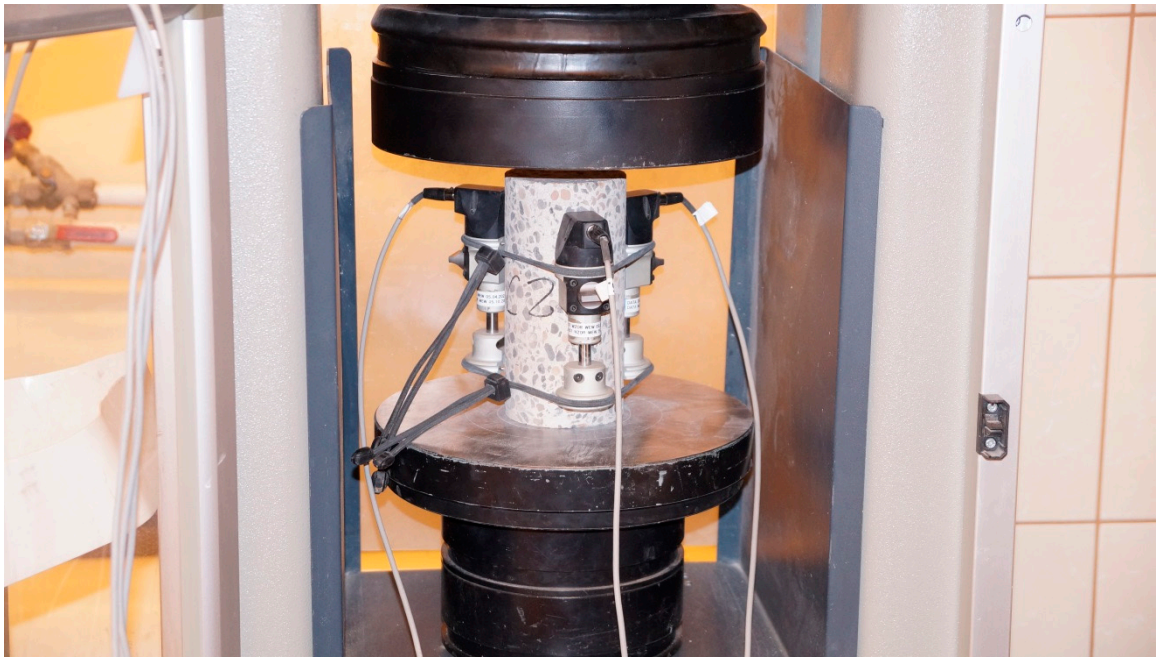
Figure 5. The device used for testing the modulus of elasticity.
