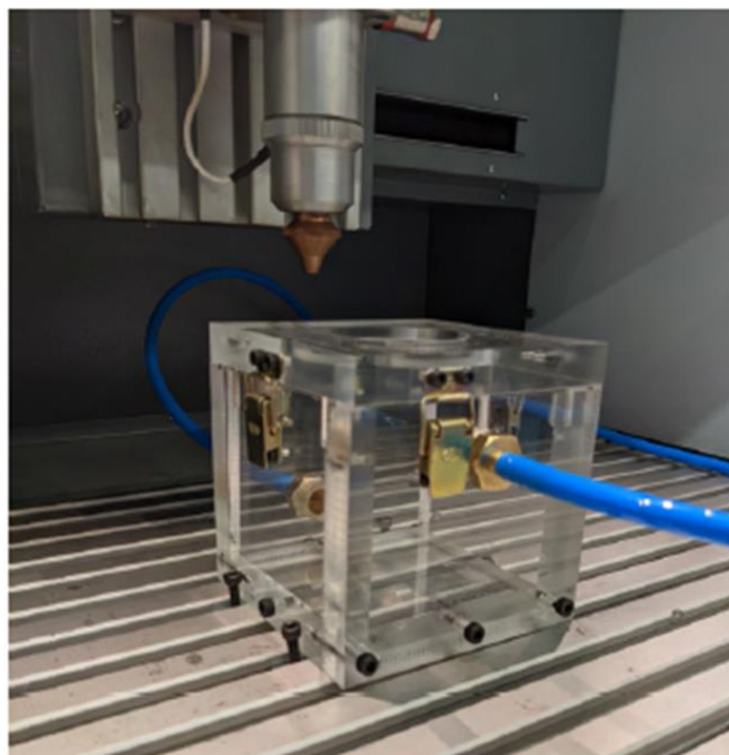
Figure 2. A custom-designed gas chamber.
