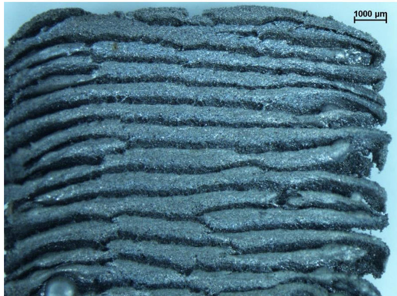
Melt pool image of the single-layer sample processed at 40 W, displaying a more robust structure with distinct melt pool lines and significantly fewer balling defects, although balling is observed at the edges where the laser beam changes direction.
