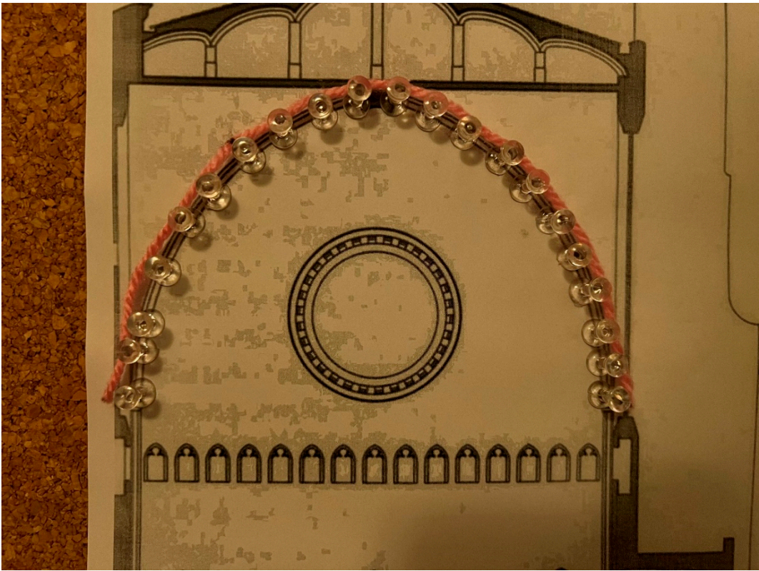
Figure 11. Close-up view of the apex and springing points, with the string adapting to the vault's contour (photograph by the author).
