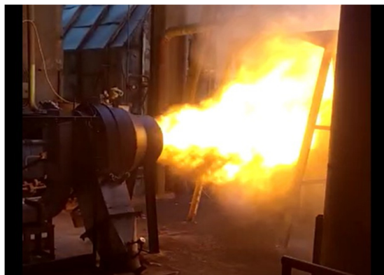
Figure 9. Flame extending up to 4 meters at a coal feed rate of approximately 3000 kg/h.
