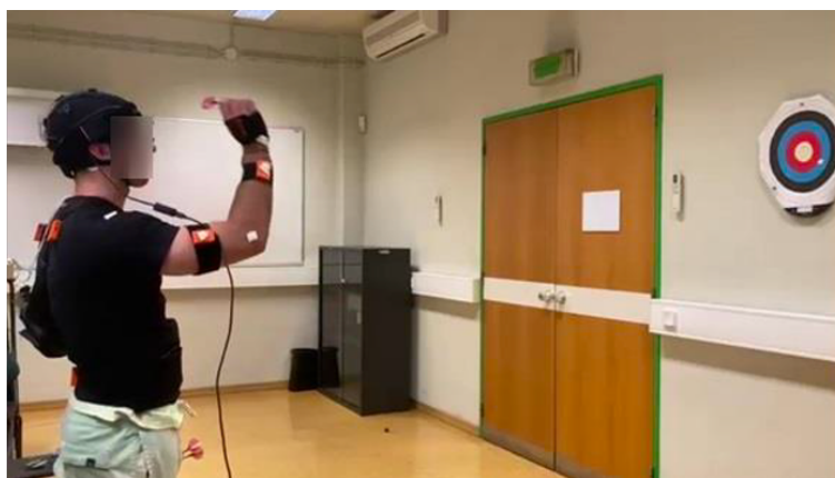
Figure 2. Experimental setup featuring the target and a participant equipped with wearable sensors during a trial. Sensors were placed on the participant's hands, forearms, arms and shoulders of both limbs to capture biomechanical data, while the participant performed the dart-throwing task. This configuration allowed for real-time monitoring of movement patterns, posture, and throwing dynamics.
